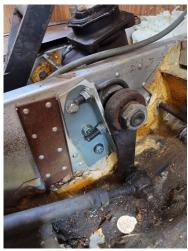
an idea to put a piece of aluminum angle and 2" exhaust clamp on the right side of the gear box housing where the shaft comes out to stop the twisting. Now everything is good.
