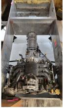
with 5-speed automatic are installed in the engine bay.
