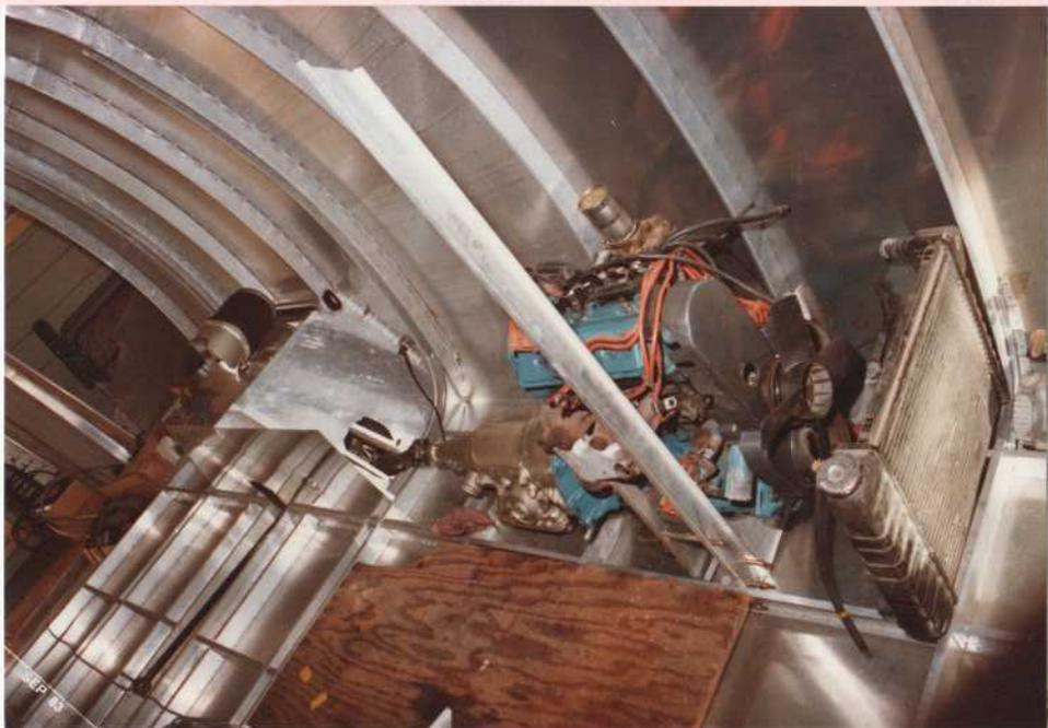
Side mounted Chevette engine with radiator.
