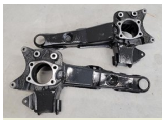
The modified part welded to the Corvair trailing arms.
