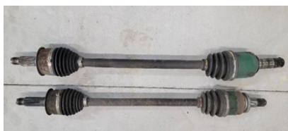
Top is the front axle; bottom is the rear. I will be using the right side of the top one welded to the left side of the bottom one.
