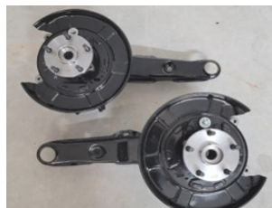
The bearing and brake mounting plate in place.
