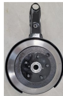
Trailing arm assembly with the 12.5" disc. These will pair nicely with the 12.2" Wilwood discs I have in front.
