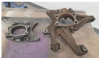
Modified bearing/ brake mount
