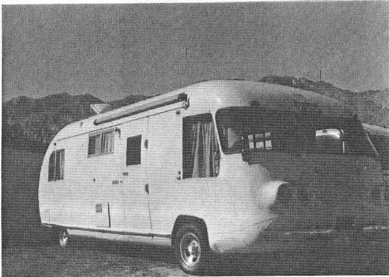
MEL'S 24 FOOTER #200. NOTE THE STRIP THAT RUNS DOWN THE FORWARD WHEEL WELL TO THE REAR. ALSO THE EARLY FORD ECONOLINE HEADLITE BEZELS
