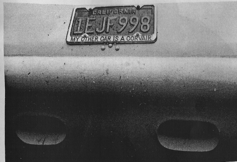
FRESH AIR VENTS UNDER THE FRONT BUMPER ON #326 DESIGNED BY HAROLD WASHMUTH
