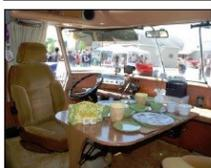
Thanks to its rear engine design the dining table on the Ultra Van was between the driver and passenger's seat.
