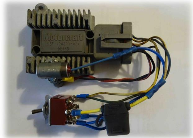
The module heat sink is about three inches square with about two inches more for the connector. The heat sink is about an inch or more tall.
