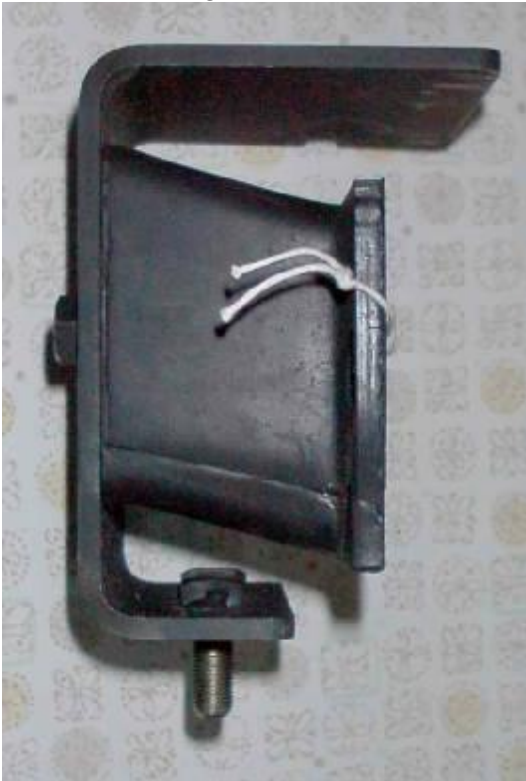
Original "redesigned" motor mount as it was received from Clarks.
