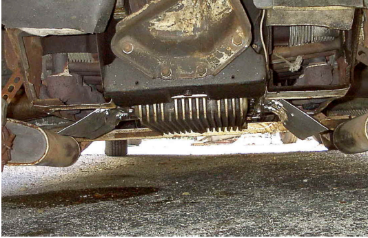
Doors partially open air blows to side Mufflers being lower protect the doors
