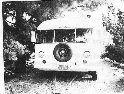
Here sits Ultra Coach , ( not ultra Van ) S/N 294 in the rear driveway of Hal and Tote Pickering's New Mexico Rancho on the morning that we took possession of it. Those bumpers are / were steel units bolted to heavy aluminum channel which was then riveted into the structure. They have been removed so that Phil Finch can have a Norm Helmkey " Smiley Face " on the front .
