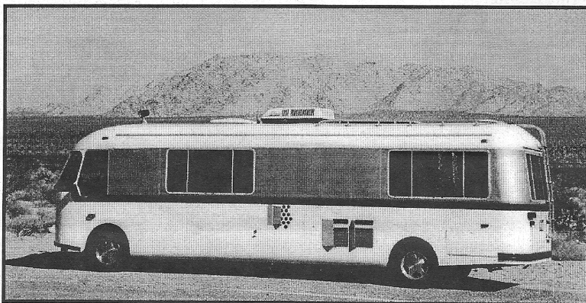
Note the radiator out let on the lower side ahead of the rear tire. There is another radiator laying flat under the forward side window. The engine is just behind the forward side window. Jim says it runs cool with the two radiators.
