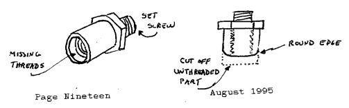
TECH TIP NO. 95-25 SUBJECT Installing Teflon Valve Stem Seals UV MANUAL SECTION 13 PAGE 13-23 AUTHOR Norm Helmkay #486
