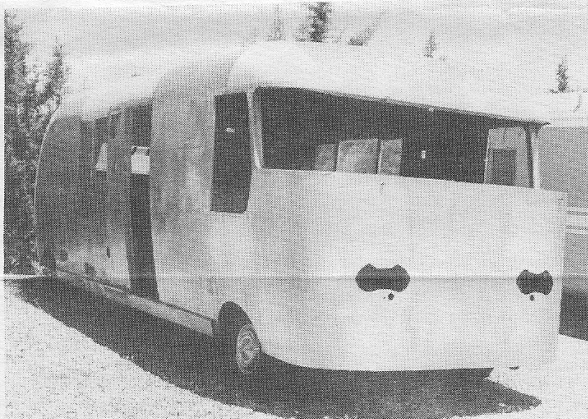
Right side of #101 showing new sheet metal, minus glass.
