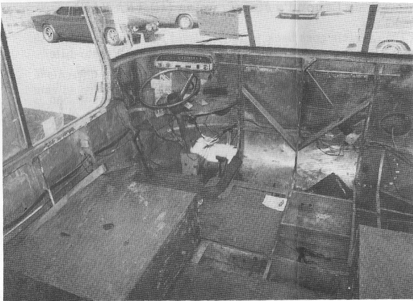
Forward Driving Compartment. Note windshield wiper uses one motor with a shaft to drive the right blade.
