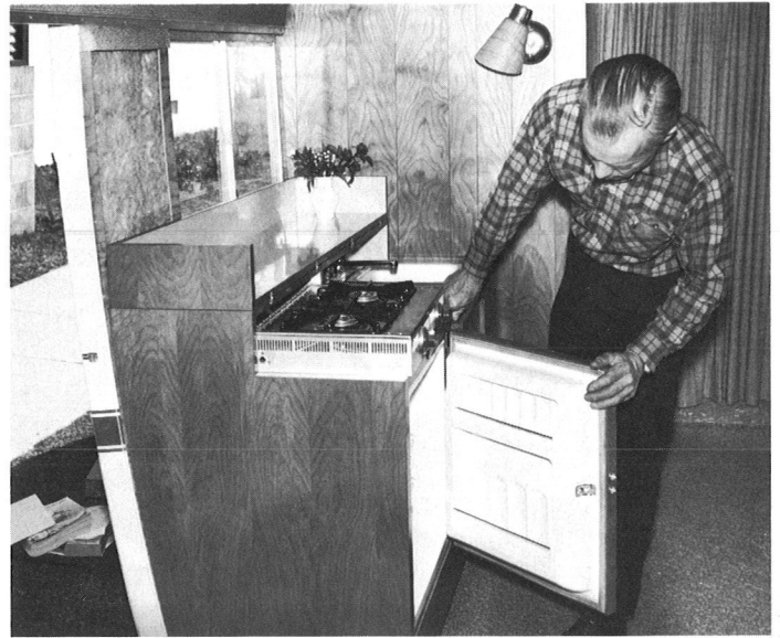
Another interior view of #101 shows designer David Peterson opening the gas refrigerator under the propane stove. Note the sink behind the stove. The cover swings over and covers the stove and sink. This photo was taken in 1961 at Peterson's home.
