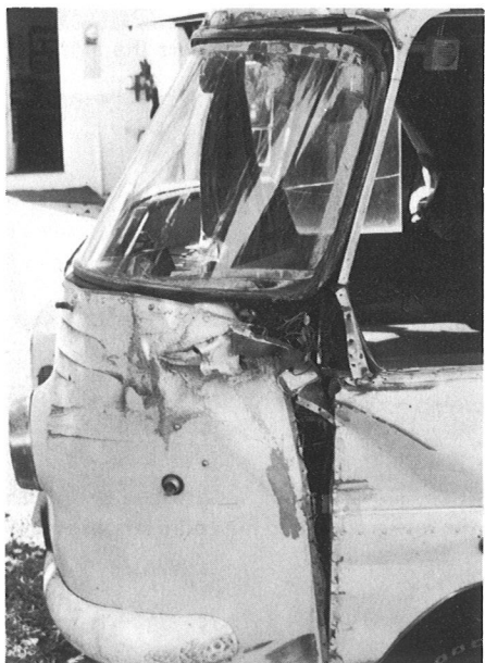
This driver's side photo of Barden's van shows how the entire front section was pulled forward in the accident.
