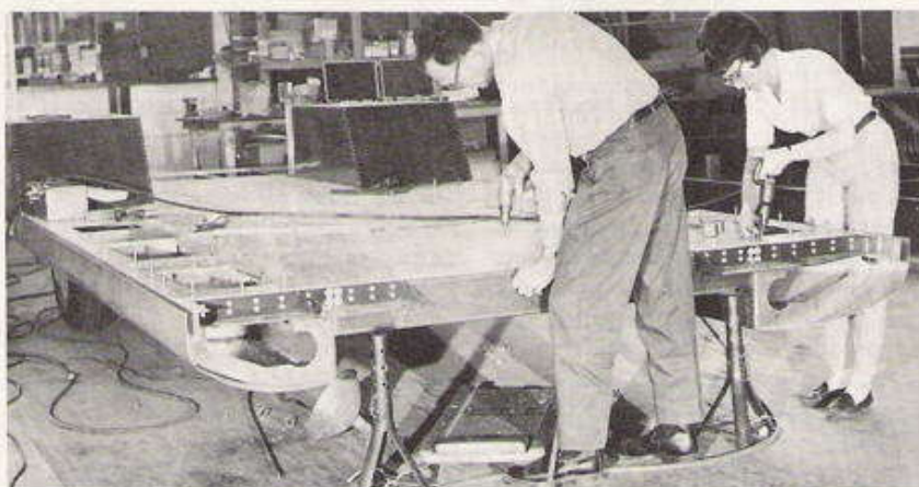
▲ The rolled and welded aluminum rocker panels, have out-riggers and bulkheads attached as shown. Gasoline, holding and fresh water tanks go underneath for a LOW center of gravity.
